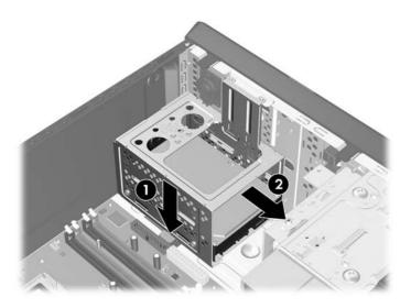
8. Lift the hard disk drive cage out of the chassis.
